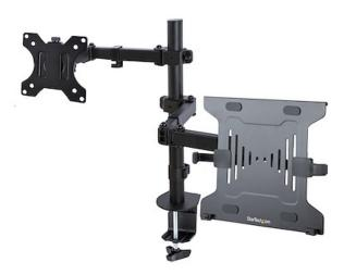
Increase your desk space and add versatility and ergonomics to your work/home setup with this VESA-compatible laptop and monitor desk mount. The laptop tray (11.8x11in / 300x280mm) is large enough to hold a laptop between 9.4-16.5in (240-420mm) wide, 1in (25.4mm) thick, and up to 10lbs (4.5kg). The monitor arm allows you to mount a VESA compatible (75x75mm or 100x100mm) display up to 32in with a maximum weight of 17.6lbs (8kg).
